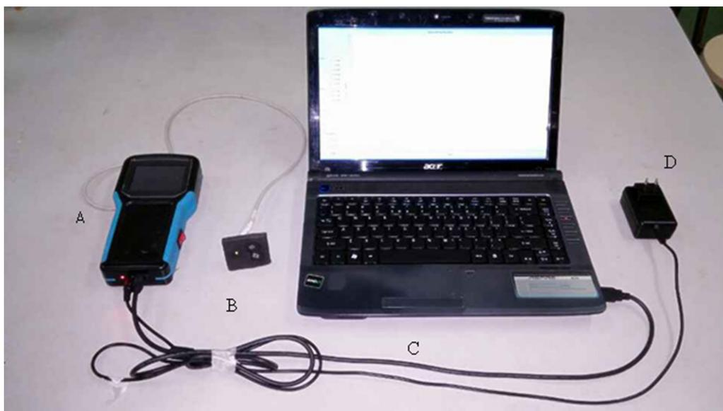
**Figure 2.** A. Probe; B. data acquisition and control module; C. calculation module; D. power module.
